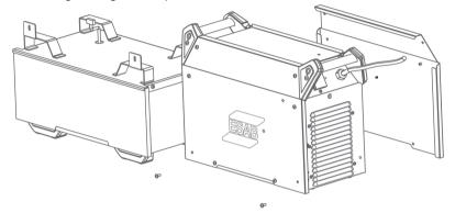
c. Place the power source on the adaptor and connect the cable through the bottom plate to PCBA. Plug the connector into P6.
