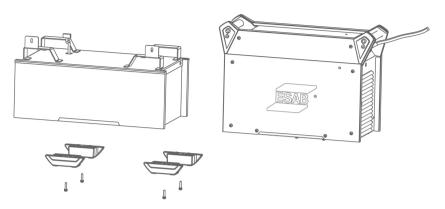
b. Remove the screws holding the left side panel and remove the panel. Remove the two screws holding the right side panel.
