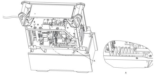
d. Assemble the power source and the adaptor with the screws.
