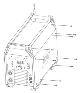
3 Clean the right side of the power source, using dry compressed air with reduced pressure.
